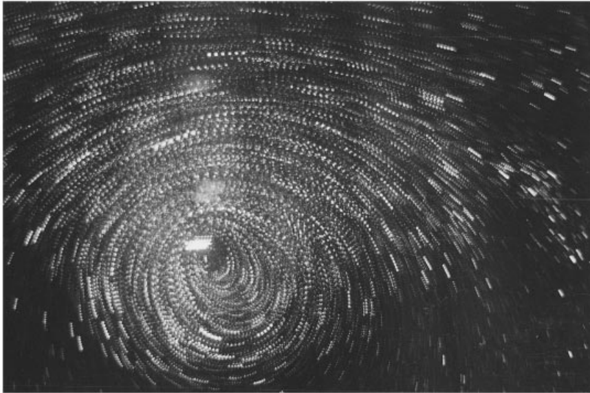
FIGURE 13. Image of an initially circular turbulent vortex ring after entraining 1100\ \mu\text{m} bubbles. The flow is from right to left as the images were recorded with Camera B.
